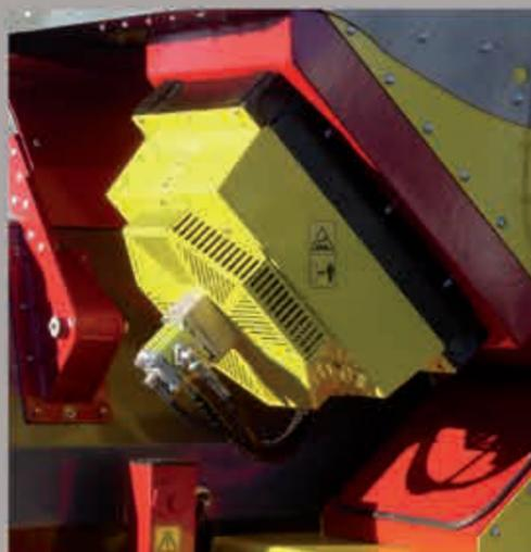
**SCAMBIATORE DI CALORE CON VENTOLA IDRAULICA**
